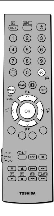
First press and hold the  $\oplus$  button until the video input mode list appears on the screen, then press the  $\checkmark$  or  $\land$  and **OK** buttons in order to select the PC input mode (see page 29).
